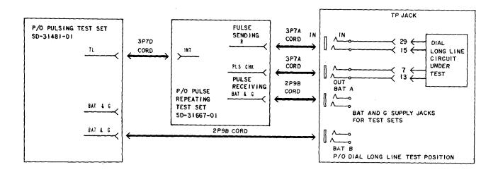
Fig. 1—Test Equipment Connections
